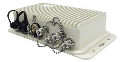
The new SensX EXTREME rugged reader is Sens-Thys' highest performance RFID reader enclosed in the industry's highest rated IP67 industrial and weather-tight chassis for harsh environments. Operators can now install RFID reader networks in places where traditional readers have previously not been suited.
